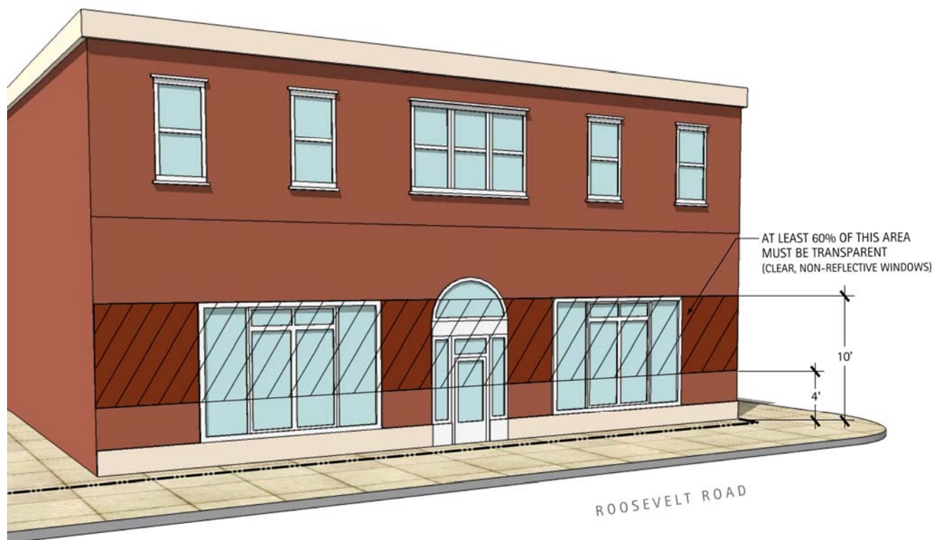
Figure 19: 50% to 60% Transparency and Entrance Doors Adjacent or within 15 feet of the Build-to-line (Transparency measurements between 4 feet and 10 feet above grade.)
